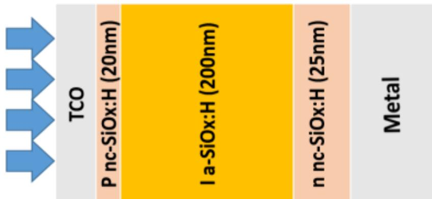
Fig.1: Schematic structure of a-SiO<sub>x</sub>:H based thin film solar cell.
